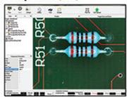
Optical Color Inspection is a feature which provides more flexible and robust color detection for devices with color. It can be used to inspect colour dot, chip absence / presence, solder beading, colored ring inspection etc.
