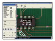
OCR allows the user to program V510 system to read text printed on the body of a component. This algorithm provides multiple fonts inspection capability without any template learning.
