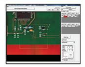
Flexible Universal Fiducial provides flexibility of fiducial point assignment by using universal feature point (test point, wire line or even empty pad) when there is no fiducial point on the interested FOV. It would also help in PCB warpage compensation.
