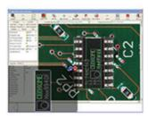
eOCV is capable to detect wrong part and wrong orientation efficiently. This algorithm is able to verify any character shape on the component.
