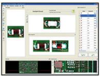
A clear and user friendly defect verification tool allows the operator to review inspection result easily and accurately with SPC capability. Colour scaling is used to illustrate the component height measurement.
