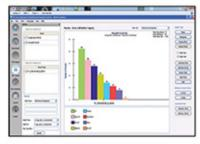
A tool for acquiring data from multiple ViTrox optical inspection systems and processing the data collected into meaningful statistical process control (SPC) information and charts from a centralized location, for the use of various management functions.
