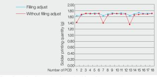
Effects from cleaning and estimated solder printing quantity: Better solder printing via filling adjust function
