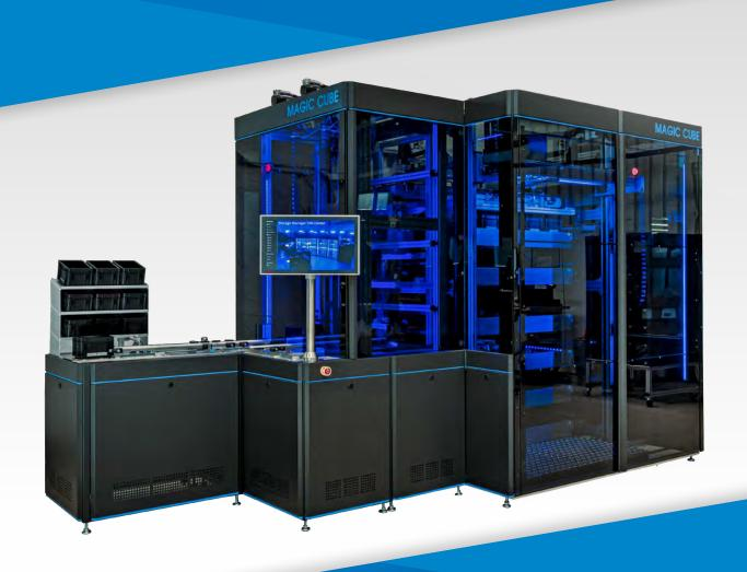
Fully automated storage and picking system for small parts, boxes, blisters and circuit boards
