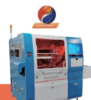
MicroCut 300 is an inline laser cutting equipment that uses non-contact cutting technology to effectively prevent deformation and stress during cutting.
